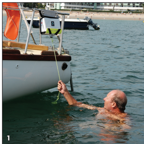
1 Pull the cord to open the flap of the reboarding ladder case.
