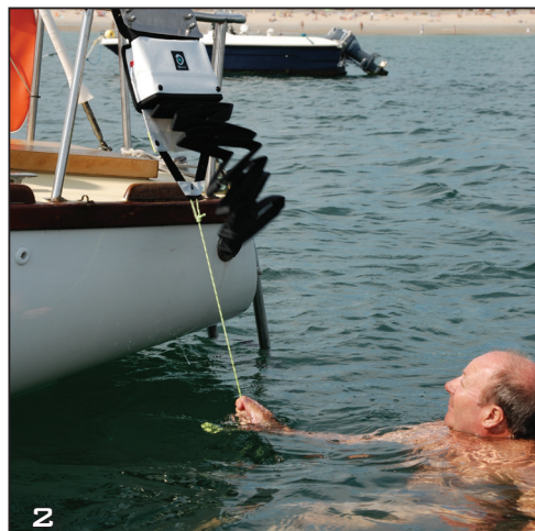
2 Once the flap is opened, the ladder deploys automatically.
